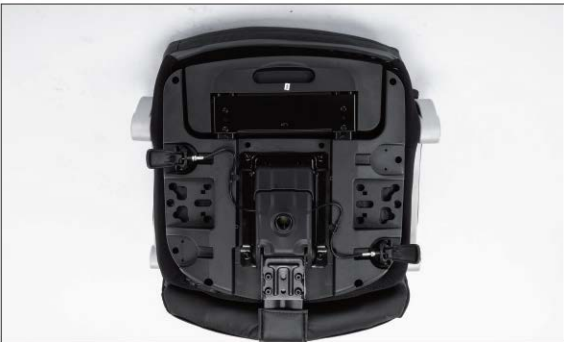
Weight Balance Mechanism by Cable Control
